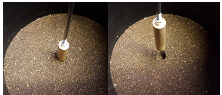
TML Penetration Test bits with soil sample material
